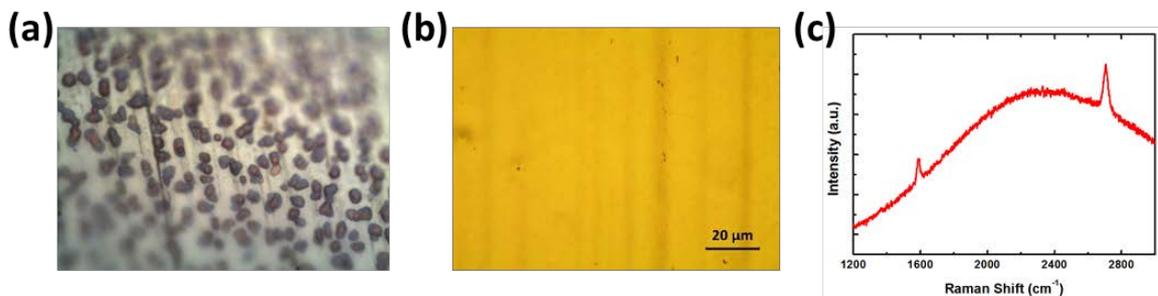
Figure 1. (a) Optical microscope image of partially oxidized Cu foil. (b) Optical microscope image of Cu foil covered with fully grown graphene (c) Raman spectrum of as grown graphene (on Cu foil) after growth steps.
